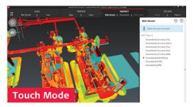
Benefit from touch-friendly guided workflows to connect to Leica Cyclone field applications, to do as-built analysis and create real-time colour maps and reports to support rapid decision-making in the field.
